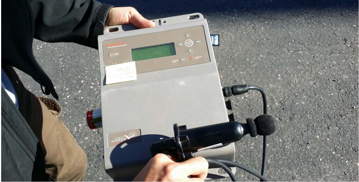
Figure 3. A Wildlife Acoustics SM3Bat recorder and SM3-U1 microphone used for monitoring bats at stationary points. Note the battery compartment on the left side and the memory card and antenna ports on the right side. (NPS)
